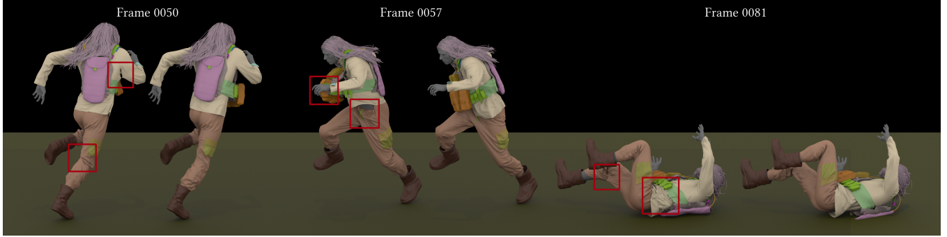
Figure 1: Character animation often suffers from nonphysical pinching (e.g., at armpits and knees) which can destabilize costume simulation (left, red boxes). Our proposed methods (right) stabilize collisions without changing the animation. ©Wētā FX.
